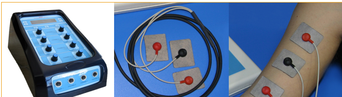
Fig. 1a, 1b, 1c - Neuromuscular measurement device NM4, superficial electrodes and example of placement of electrodes.
