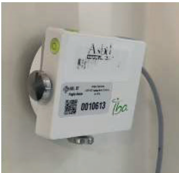
Fig. 2 - Arc IMRT angular correction sensor
