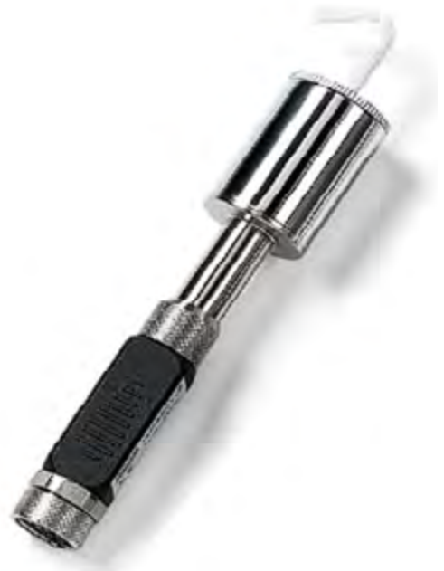
Figure 2. Naturally ventilated wet-bulb temperature probe
