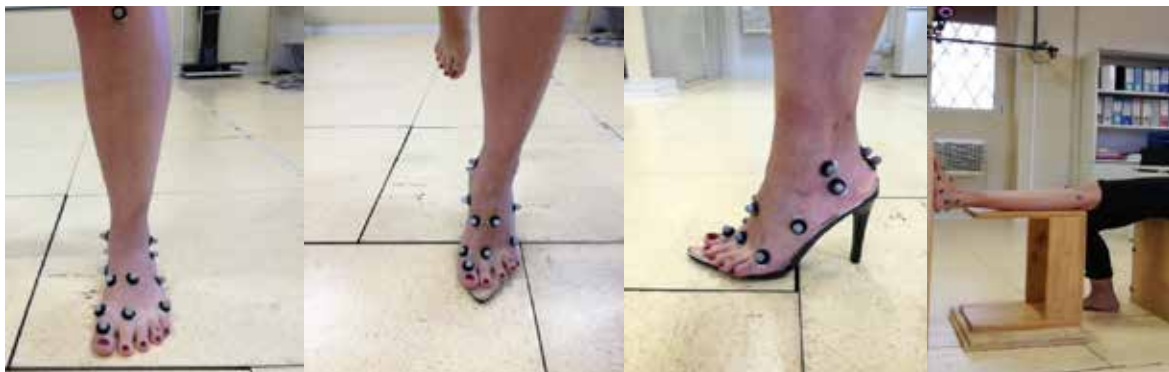
Fig 9-10-11-12 – From top left, clockwise : Gait Analysis acquisition with left foot under load; with shoe with heel (front view); with heeled shoe (side view); unloading.
